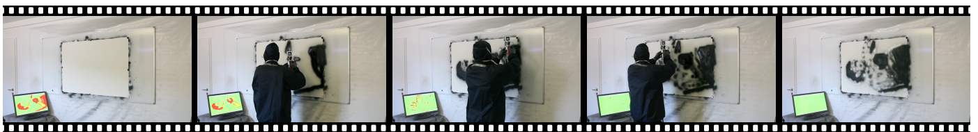
Figure 3: For our physical experiments, the user waves our modified spray can before a 1.5 m 2 canvas. The monitor to the left shows the potential residual for the current color, as well as the spray can location, helping the user to position himself and to find areas to improve. See the accompanying video for a full painting session.
